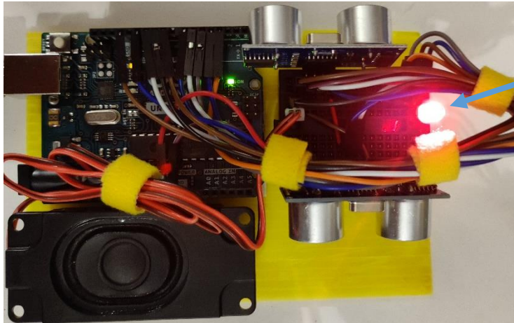
Figure 10 - Theremin assembled using only one breadboard and only one loudspeaker
